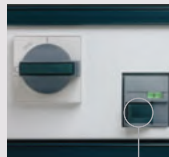
Operation error protection enabled (main switch 0)
