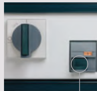
Operation error protection disabled (main switch I)
