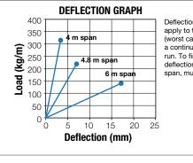
Deflections shown apply to the end bays (worst case) of a continuous ladder run. To find deflection of a single span, multiply by 2.5.
