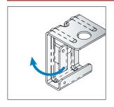
Rotate the retaining tab into the open (horizontal) position.
